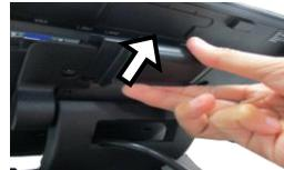
6. Properly insert the cable into the correct port on the bottom I/O plate.
