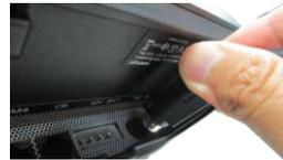
7. Neatly arrange your cable. Then, make sure the cord can be held into place and passed through the cable exit after sliding back the cable arrangement cover.
