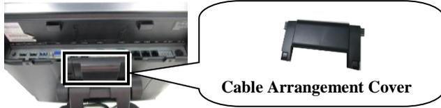
5. Remove the cable arrangement cover by pushing it up in the direction shown by the arrow.
