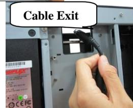
6. Neatly thread the cord along the bottom edge of the PoweredUSB compartment (1), and then use the cable tie to hold the extra cable (2) as shown in the figure.
