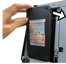
3. After pushing the power adapter up to the top, place two brackets separately on the top and bottom sides of the power adapter compartment as shown in the figure. Then, fasten two brackets with four fixing screws.
