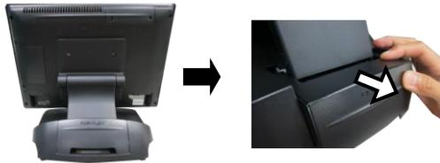
2. Pull outwards the locking levers with your forefingers and then remove the neck cover in the direction shown by the arrow.
