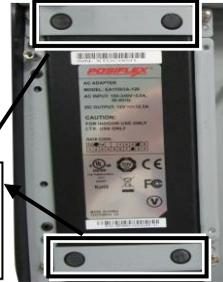
4. Before threading the cable through the cable exit, loosen two fixing screws for the bracket of the PoweredUSB compartment. Then, slide the bracket in the direction shown by the arrow to remove the bracket.
