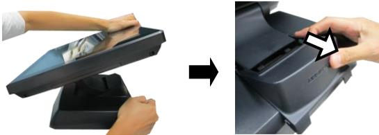
6.2 Support the screen with one hand holding onto its bottom edge. While pulling the lever backwards, release the lever back to the point above the upper hook as shown in the figure.
