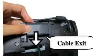
8. Have the screen tilt all the way down, and then push the neck cover back into place, and then place the cable cover back.
