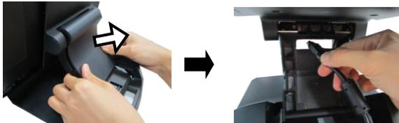
4. Tilt the terminal up enough to have the bottom I/O plate towards you. Locate the cable arrangement cover as shown in the figure.
