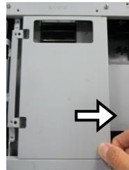
5. Pass the cable of the power adapter through the cable exit and then connect it to the port on the I/O plate of your POS system. (Please refer to **Routing and Arranging Cables** section to thread the cable, according to the model of your base.)
